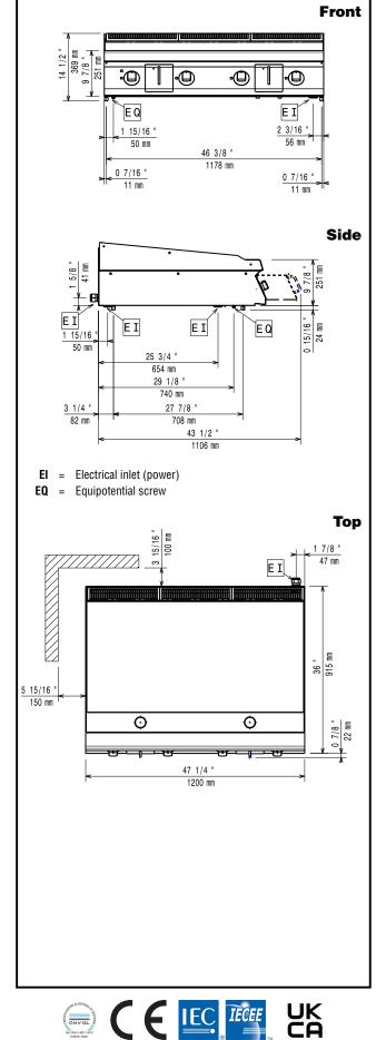
Modular Cooking Range Line EVO900 1200mm Electric Fry Top HP, Smooth Scratch Resistant Chromium Plate The company reserves the right to make modifications to the products without prior notice. All information correct at time of printing.
